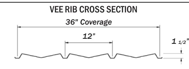
NOTE: ALL PANELS FORMED FROM LIGHT GAUGE METAL MAY EXHIBIT WAVINESS, ALSO KNOWN AS "OIL CANNING," COMMONLY OCCURRING IN, BUT NOT RESTRICTED TO, FLAT PORTIONS OF A PANEL. THIS INHERENT CHARACTERISTIC IS NOT A DEFECT OF MATERIAL OR MANUFACTURING AND IS NOT CAUSE FOR REJECTION.
