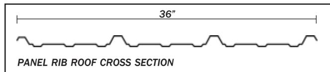
**NOTE: ALL PANELS FORMED FROM LIGHT GAUGE METAL MAY EXHIBIT WAVINESS, ALSO KNOWN AS "OIL CANNING," COMMONLY OCCURRING IN, BUT NOT RESTRICTED TO, FLAT PORTIONS OF A PANEL. THIS INHERENT CHARACTERISTIC IS NOT A DEFECT OF MATERIAL OR MANUFACTURING AND IS NOT CAUSE FOR REJECTION.**
